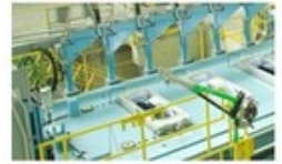
Very Wide Fuselage Skin to save Longitudinal and Circumferential Joints at OEM
