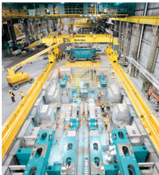
Our Very Thick Plate Stretcher, which will make plate for the aerospace industry's largest high-strength monolithic wing ribs, comes online in 2017.
