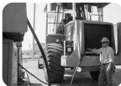
Refueling with B20 soy-based biodiesel
