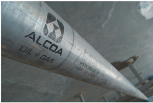
FarReach alloy drill pipe
