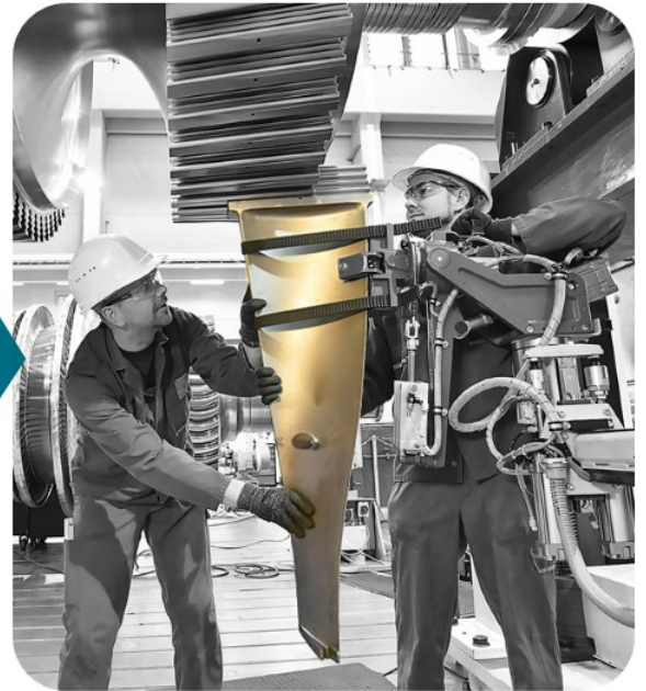
Howmet Produces Large DS Blades Greater Than 3 Feet Long
