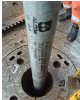
Aluminum Alloy Drill Pipe offers light weight yet high strength.
