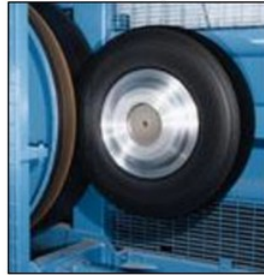
700,000 miles simulated - 2X normal loading to test durability
