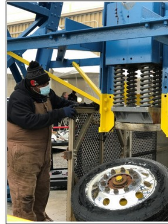
2,200 Lb weight dropped from 20 feet to test impact resistance
